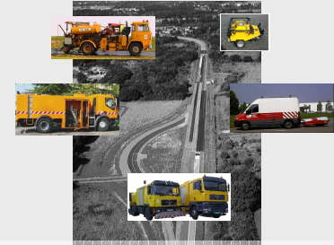
Comparison of European friction measuring machines on the reference test tracks at Ifsttar Nantes.
